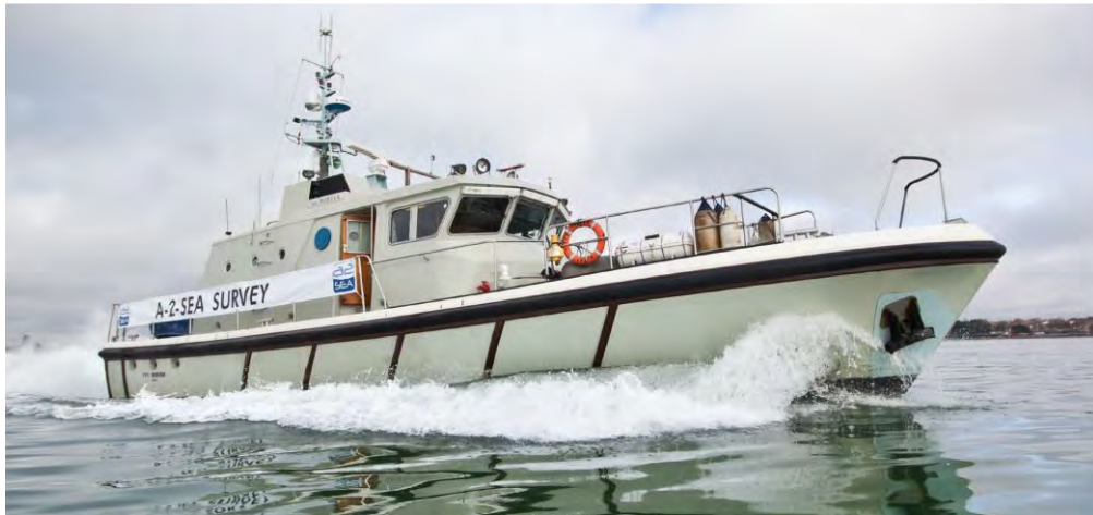
Figure 4 - FPV Morven – Survey vessel used to undertake baseline benthic grab and DDV surveys
